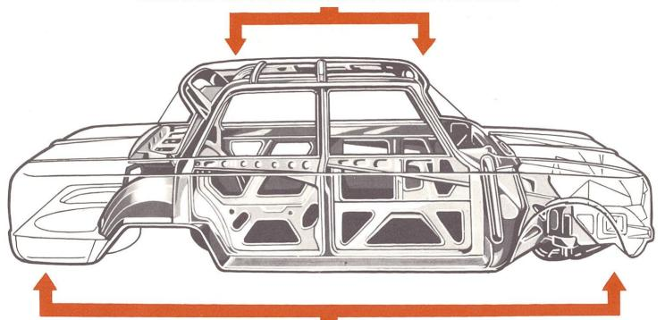
THE STRUCTURE OF THE ENGINE COMPARTMENT AND THE LUGGAGE BOOT BECOMES LESS RIGID TOWARDS THE EXTREMITIES OF THE VEHICLE IN ORDER THAT THE EFFECT OF A COLLISION SHALL BE ABSORBED AND DEADENED.
