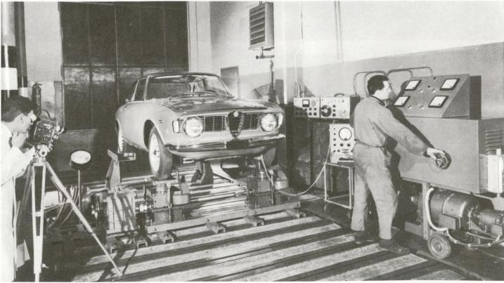
HE BOUNCES AND BUMPS ALONG - The car is mounted on pecial test bed that can give to the wheels the same rough atment they would receive if driven over an unmade road. The cks are then recorded. The tape is connected to special equip-
