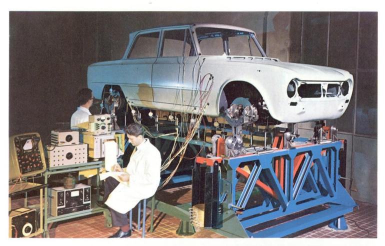
FAILURE SHOOTING - For this test the body shell is fixed to a bench and loads are applied to certain pre-determined areas. By means of strain goges attached to the most critical points of the bodywork any yielding si discovered.
