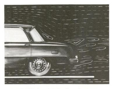
NOT LIKE THAT - A rounded tail profile would leave in its wake large vortices tending to build up towards the front of the car. This would slow it down and increase petrol consumption.
