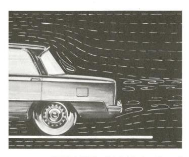
**THAT'S BETTER** - A knife-edged profile would definitely produce less turbulence towards the front of the car. The wake now is narrower than in the previous example.
